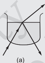
Fig. 1.6. Observing total internal reflection in water with a laser beam (refraction due to glass of beaker neglected being very thin).
